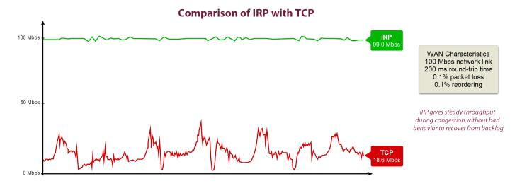
Intelligent Retransmission Protocol (IRP) guarantees delivery by efficiently retransmitting dropped packets without violating bandwidth constraints. As opposed to TCP, IRP does not spend time searching for an optimal rate, nor does it interpret packet loss as a signal to slow down. The result is reliable network transport that is many times faster than TCP.
